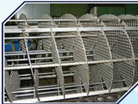
Helical Tube Bundle Skeleton
