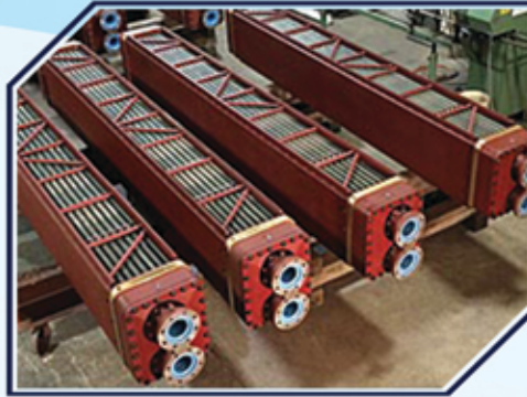
Generator Air Cooler
