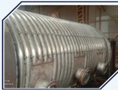
Blender Shell With Limpet Coil
