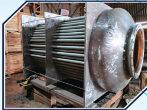
Coke Oven Gas Cooler
