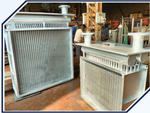
Nitrogen Regeneration Cooler
