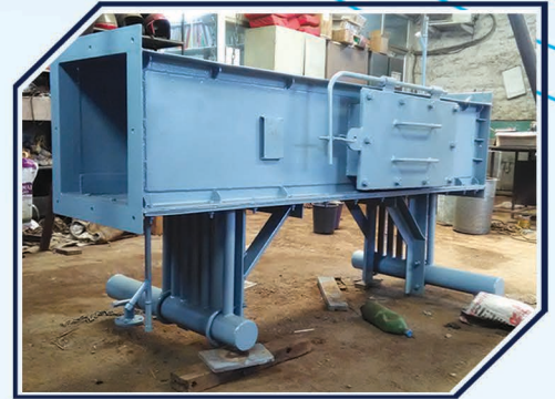
Flue Gas Cooler
