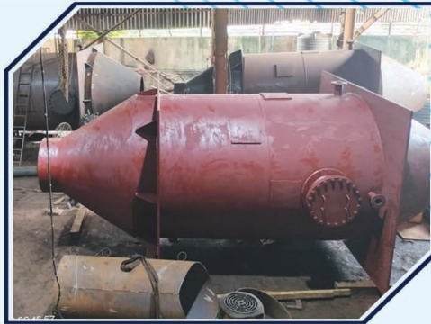
Heat Exchanger for Tar Producer Gas Plant
