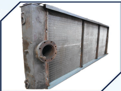
Radiator for 100 MVA Generator
